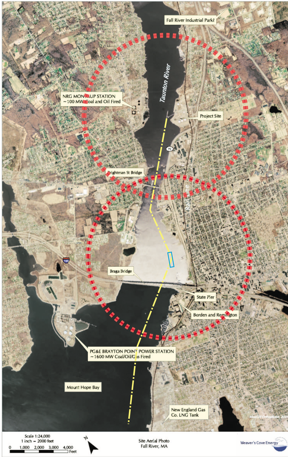
Figure 3: The path of a tanker approaching the proposed LNG terminals (yellow dashed line) and the radiation danger zones for a spill at two locations along this path.
